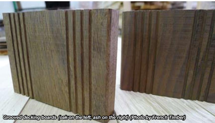
*Grooved decking boards (oak on the left, ash on the right) (Photo by French Timber)*
